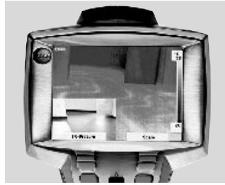
Image-in-image function for easier orientation and simple documentation
